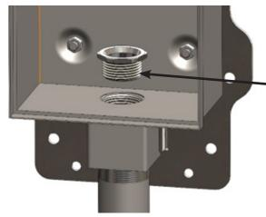
Install 1" Chase Nipple Through Disconnect, Into the Mounting Block
