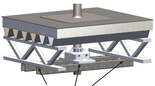
Bolt Strut to the Mounting Base Using 1/2-13 Threaded Holes and Secure Strut to Roof Structure.
