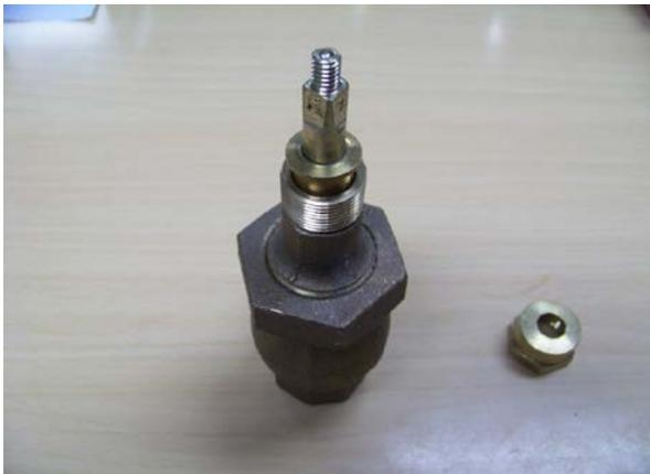
6. Replace bushing and packing nut. Tighten packing nut hand tight with an addition  $\frac{1}{2}$  turn.
