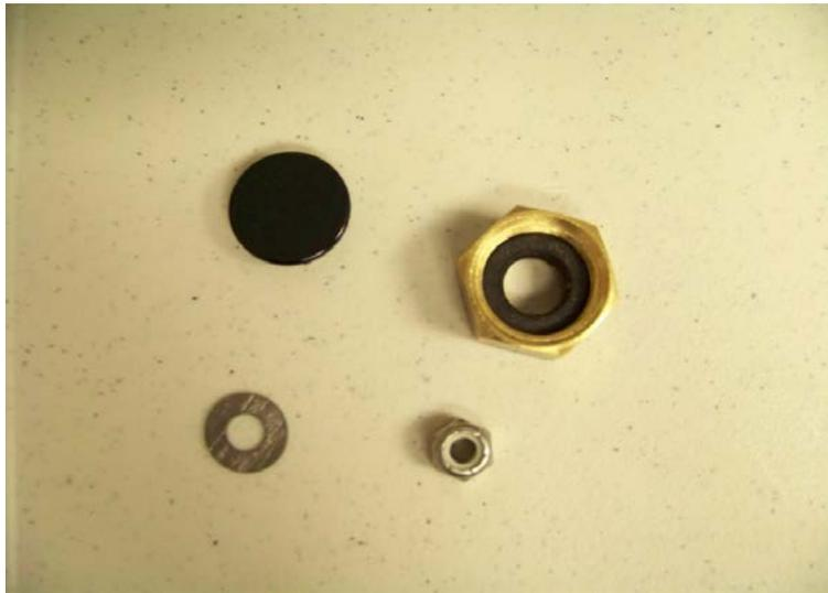
5. Replace packing nut with the one supplied in your repair kit.
