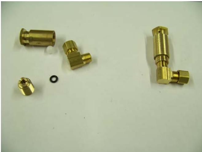
2. Blow air into the holes of the assembly to dislodge any debris that has accumulated around the nylon ball. This will cause the ball not to seat properly thus allowing water through.
