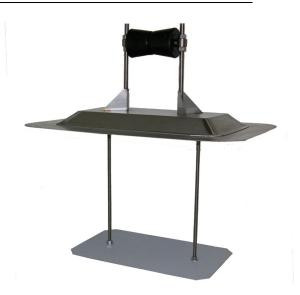
**Composition:** Grade 304 Stainless Steel with continuously welded seams and rounded edges to prevent incidental damage to the roof surface and a 3" perimeter deck flange provides flashing to the roof deck.
