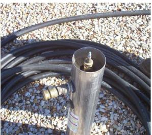
2. Loosen and remove the  $\frac{1}{4}$ " lock nut and washer inside the cavity.
