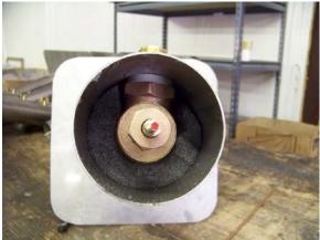
3. Lift Dome Handle to expose inner cavity of Shroud
