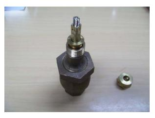
6. Replace bushing and packing nut. Tighten packing nut hand tight with an addition ½ turn.
