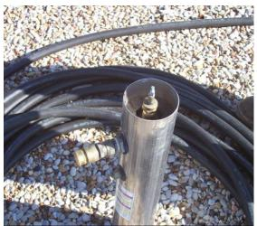
2. Loosen and remove the  $\frac{1}{4}$ " lock nut and washer inside the cavity.
