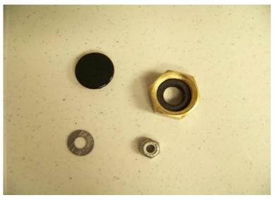
5. Replace packing nut with the one supplied in your repair kit.
