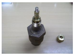
6. Replace bushing and packing nut. Tighten packing nut hand tight with an addition ½ turn.
