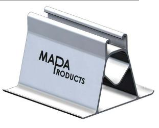
Standard Composition: Extruded Aluminum with integrated 1 5/8" shallow strut, Solid flat base with rolled edges. Available lengths pre-cut up to 10'. 100% recyclable material. Made in USA.
